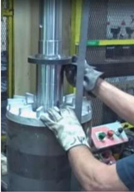
Figure 4. Measuring the correct tolerance.
